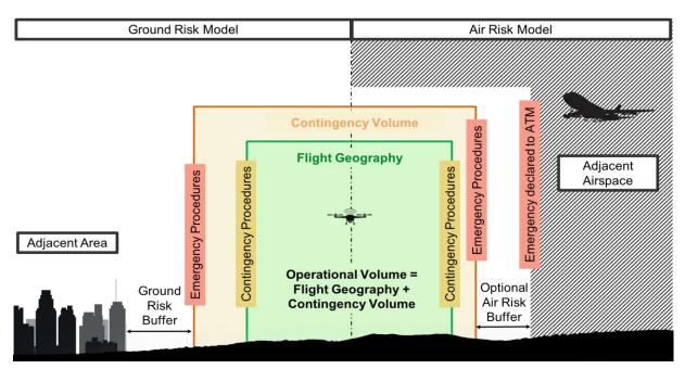
Figure 2 — Graphical representation of the SORA semantic model
